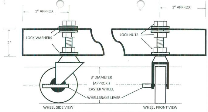
FOUR (4) PIECES THREADED BOLT TYPE SWIVEL CASTER WHEEL WITH BRAKE 3" DIAMETER
